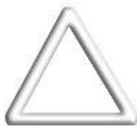
Figure 4.7 Tactile warning or danger in the form of a raised triangle.
